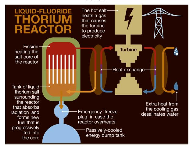
**THORIUM MOLTEN SALT REACTOR:** Forgotten war technology could safely power Earth for millions of years. Here's why we aren't using it <a href="http://www.businessinsider.com/thorium-molten-salt-reactors-sorensen-lftr-2017-2">http://www.businessinsider.com/thorium-molten-salt-reactors-sorensen-lftr-2017-2</a>
