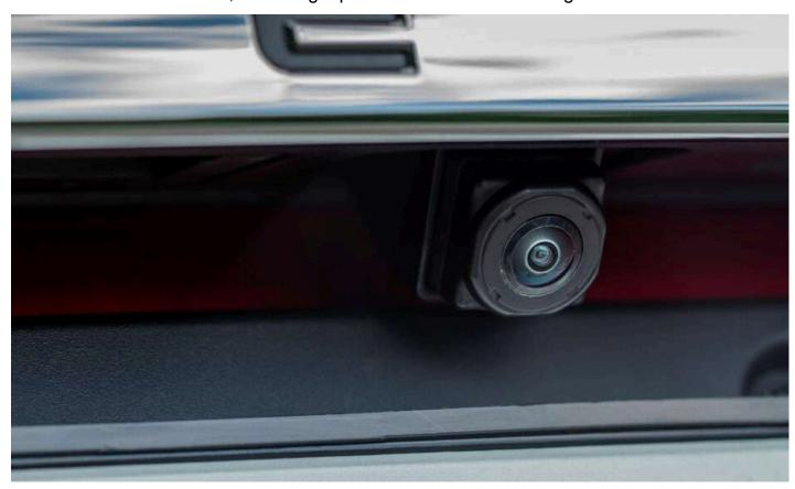
technology. These cameras, seamlessly powered over a single coaxial cable, ensure bidirectional control data and power transmission alongside high-speed video delivery. With lower latency and higher frame rates, Vadzo's GMSL cameras operate seamlessly up to a distance of 15 meters from the host processor.
