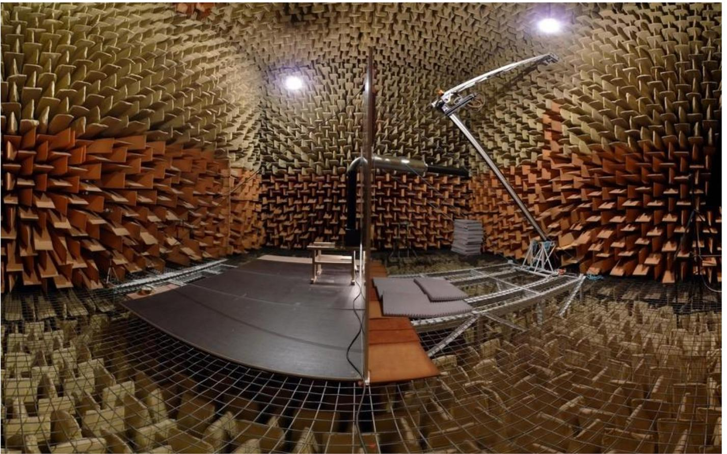
Chamber mass is estimated at 600 tons, and the same "cube" is set on vibration isolation supported on the 100 springs, which limit the transmission of vibrations from a nearby road.
