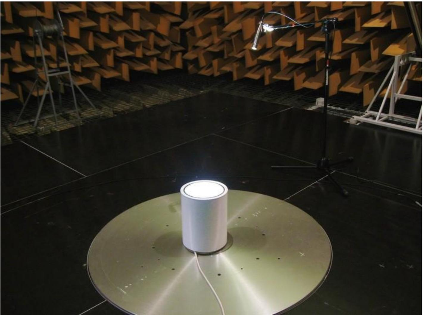
Background sound pressure level, measured in the chamber during the day is about 1.5 dBA (night time falls even below 0 dB).
