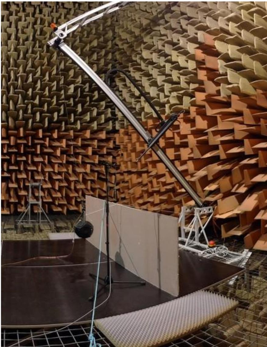
Inside the chamber is mounted keypad prototype to measure the sound power level whose capabilities have been extended to the measurement of directivity and dispersion.
