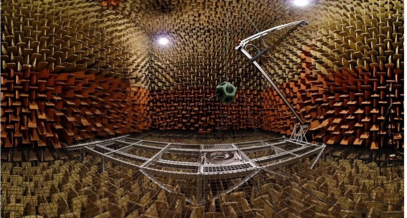
This is a special room in which you can find conditions of the free field by using special items on the walls with diffuse-absorbing properties.
