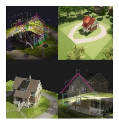
3D laser scanning is a cutting-edge technology that captures the exact size and shape of physical objects using laser light. This process involves directing laser beams at a surface and measuring the time it takes for the light to return to the sensor. These measurements are then used to create a precise, three-dimensional digital representation of the object. As Built Services utilize this technology to provide accurate documentation of existing conditions.
