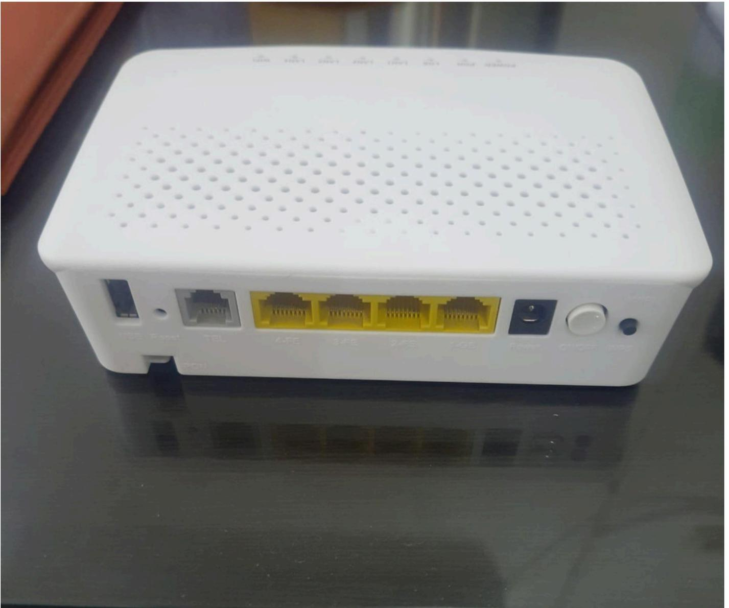
A **single band XPON router** is a type of router that uses a single wavelength of light to transmit data over a fiber optic cable. It is typically used in homes and small businesses where fiber optic internet service is available.
