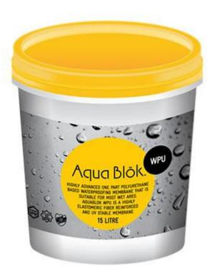
WPU / <u>AQUABLOK Waterproof</u> is based on polyurethane polymer technology that is water based. The cured membrane is a class 3 membrane with a high degree of elasticity. WPU is a single-component, premixed elastomeric waterproofing membrane for use in interior and exterior applications, as well as beneath tiled surfaces.
