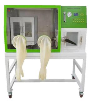
Labmate anaerobic incubator is designed for cultivating anaerobic microorganisms in an oxygen-free environment. It offers a temperature range from 3°C above room temperature to 60°C, precise control, UV sterilization, solenoid valve gas control, and a deoxidization catalyst, ensuring reliable and safe operation.
