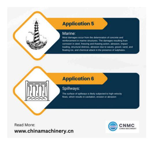
There are different fields, where **shotcrete** plays an important role and proves its good workability, compressive strength and bonding where ordinary concreting fails.
