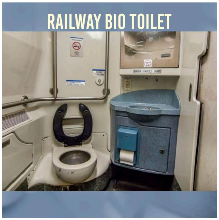
Railway bio toilet are eco-friendly as they reduce water consumption and utilize bio-digestion technology to treat waste onboard trains.
