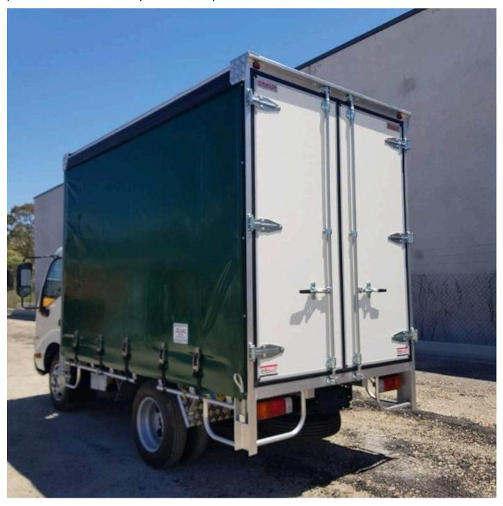
With an engineer certified and load rating floor of 980kg per pallet space, the Duralloy curtain
