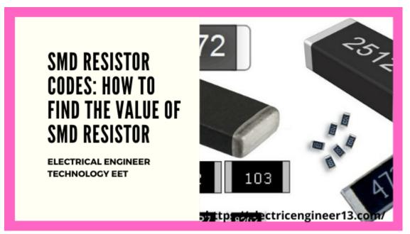
Smd resistor codes If the value of the calculator or the smd resistors is found SMD resistor: Surface mount technology SMD resistor means "Surface Mount Device" (SMT = taken by Surface Mount technology) resistor. These small chips are marked with three (3) or four (4) digit codes called SMD resistor codes to indicate their resistance... Read More »
