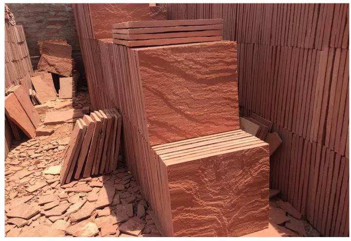
Sandstone rock is frequently naturally craggy and jagged before being levelled with gauging to create floor tiles. Sandstone tiles can be honed further to make them even smoother, flatter, and gleaming. Our sandstone tiles are frequently textured and rough, lending them a rustic and traditional appearance, making them ideal for an older home or for use in a kitchen.
