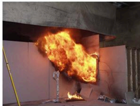
Photographs of the burn room doorway on right with PPV and the flames exiting the burn room window during the same experiment on the left.
