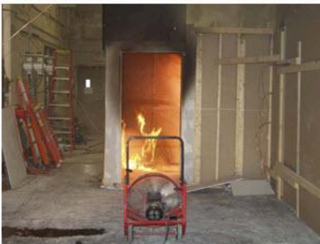
Photographs of the burn room doorway on right with PPV and the flames exiting the burn room window during the same experiment on the left.
